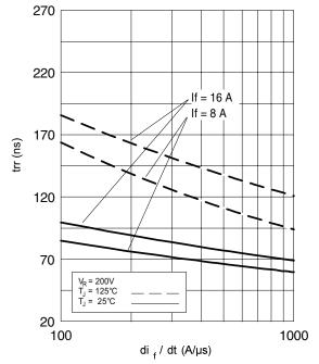
Fig. 5 - Typical Reverse Recovery Time vs. dl<sub>F</sub>/dt (Per Leg)
