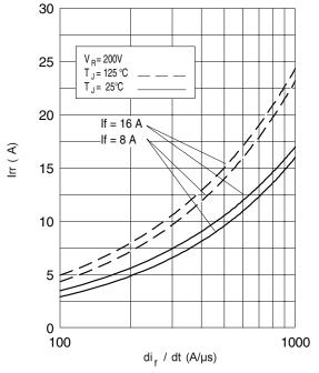
Fig. 6 - Typical Recovery Current vs. di<sub>F</sub>/dt (Per Leg)
