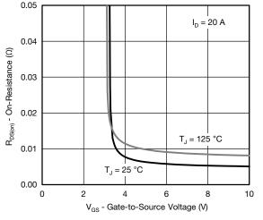
**On-Resistance vs. Gate-to-Source Voltage**
