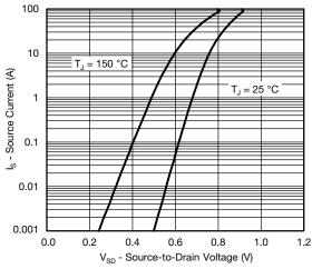
Source-Drain Diode Forward Voltage
