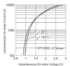
Fig. 9 - On-State Voltage Drop Characteristics
