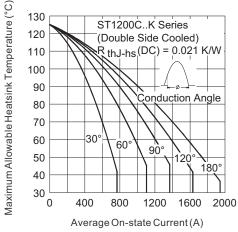
Fig. 3 - Current Ratings Characteristics
