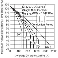
Fig. 2 - Current Ratings Characteristics
