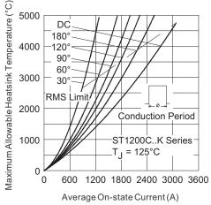
Fig. 6 - On-State Power Loss Characteristics
