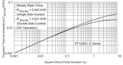
Fig. 10 - Thermal Impedance Z<sub>thJ-hs</sub> Characteristics
