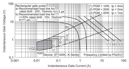
Fig. 11 - Gate Characteristics
