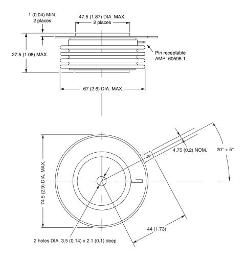
Quote between upper and lower pole pieces has to be considered after application of mounting force (see thermal and mechanical specification)
