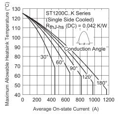
Fig. 1 - Current Ratings Characteristics
