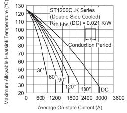
Fig. 4 - Current Ratings Characteristics
