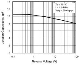
Fig. 5 - Typical Junction Capacitance
