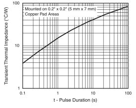
Fig. 6 - Typical Thermal Impedance
