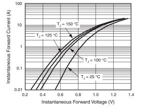
Fig. 3 - Typical Instantaneous Forward Characteristics
