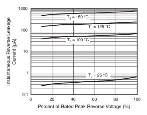
Fig. 4 - Typical Reverse Leakage Characteristics
