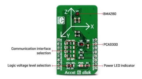
The acceleration data width is 14 bits. The filtering can be selected in several steps, with the bandwidth configuration from 8Hz up to 500Hz. The selected bandwidth configuration also affects the refresh rate, resulting in up to 64ms between consequent readings for the 8Hz setting. The unfiltered stream takes up to 0.5ms between readings.
