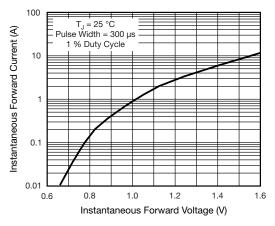
Fig. 3 - Typical Instantaneous Forward Characteristics
