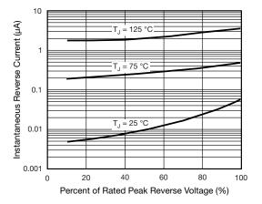
Fig. 4 - Typical Reverse Characteristics
