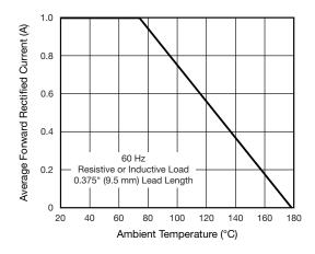
Fig. 1 - Forward Current Derating Curve
