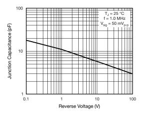
Fig. 5 - Typical Junction Capacitance
