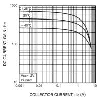
Fig1. DC current gain vs. collector current
