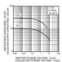
Fig 6. Collector output capacitance vs. collector-base voltage Emitter input capacitance vs. emitter-base volatage
