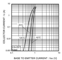
Fig.4 Grounded emitter propagation charactereistics
