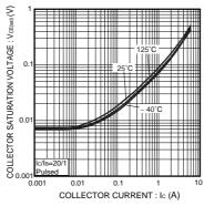
Fig.2 Collector-emitter saturation voltage vs. collector current
