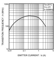
Fig.5 Gain bandwidth product vs. emitter current
