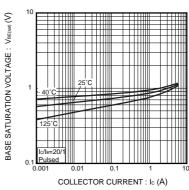
Fig.3 Base-emitter saturation voltage vs.collector current
