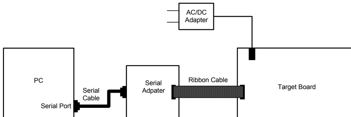
Figure 1. Hardware Setup
