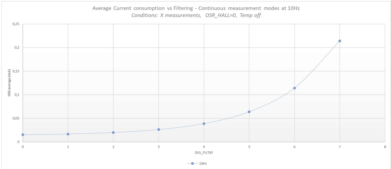
Figure 4: Average consumption vs Filtering – Continuous measurements at 10Hz – Temperature compensation off
