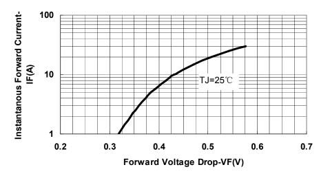
Fig.3-Typical Forward Voltage Drop Characteristics
