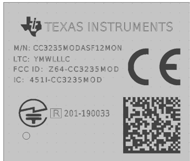
Figure 9-6. CC3235MODASF Module Marking
