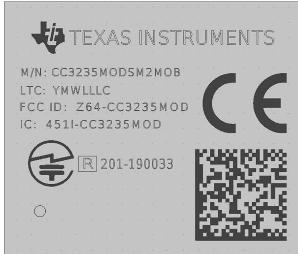
Figure 9-3. CC3235MODS Module Marking
