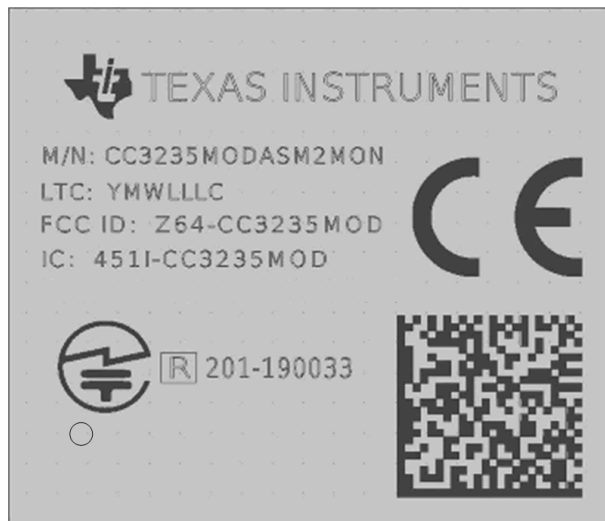
Figure 9-5. CC3235MODAS Module Marking
