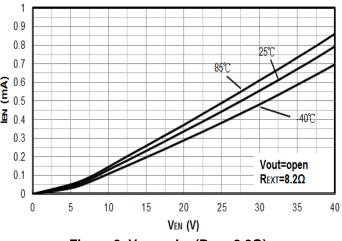
Figure 9.  $V_{EN}$  vs.  $I_{EN}$  ( $R_{EXT}$ =8.2 $\Omega$ )
