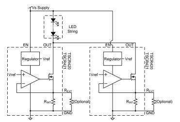
Figure 21: Application Circuit for Increasing LED Current
