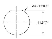
RECOMMENDED PANEL MOUNTING HOLE RECOMMENDED PANEL THICKNESS:1.6 TO 4.7MM
