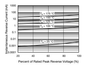
Fig. 4 - Typical Reverse Characteristics Per Diode
