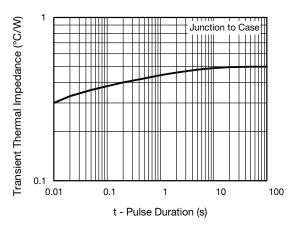
Fig. 6 - Typical Transient Thermal Impedance Per Device
