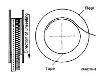
$\begin{array}{lll} d_{max} & = & 360 \text{ mm} \\ w_{max} & = & 54 \text{ mm} \\ f & = & 31 \pm 1,0 \text{ mm} \\ n & = & 45 \text{ mm (typ.)} \end{array}$
