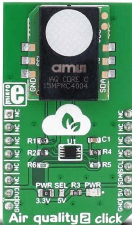
**Air quality 2 click** carries the iAQ-Core Indoor Air Quality sensor that measures VOC (volatile organic compounds) levels and provides CO<sub>2</sub> equivalent and TVOC (total volatile organic compounds) equivalent predictions. The click is designed to run on either 3.3V or 5V power supply. It communicates with the target MCU over I2C.
