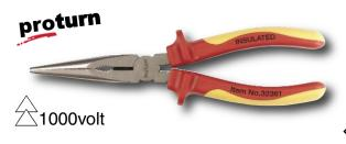
323 Proturn Insulated Long Nose Pliers. Insulation According to VDE 0682/part 201, DIN 7437, EN/IEC 60900, ASTM F-1505-01, NFPA70E, 1000 volt rated. Individually Tested. DIN ISO 5745 Pliers drop-forged from special tool steel, individually high frequency induction hardened, chrome and nickel plated, mirror polished. Proturn ergo soft grip handles for maximum comfort.
