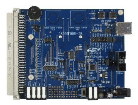
Figure .1. Example C8051Fxxx Development Board
