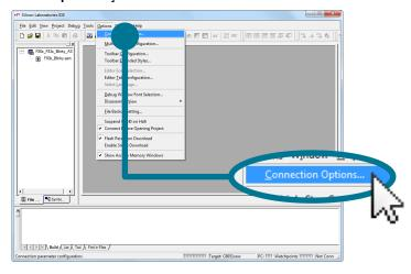
2. Select [USB Debug Adaptor] and the appropriate debug interface for the device. Devices with numbers below C8051F300 will use the [JTAG] interface, and C8051F300 devices and above will use the [C2] interface. Click [OK] to apply the settings.
