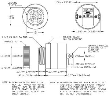
NOTE B: MOUNTING- REMOVE BLACK PLASTIC NUT AND INSERT THREADED FRINT THROUGH 1.25' HOLE PUNCHED IN PANEL, IF DRIENTATION IS NEEDED, NOTE LOCKING FLATS ON DRAVING. SCREW NUT BACK ON. DO NOT OVERTIGHTEN.
