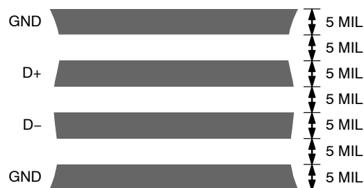
Figure 22. Typical Arrangement of Signal Tracks
