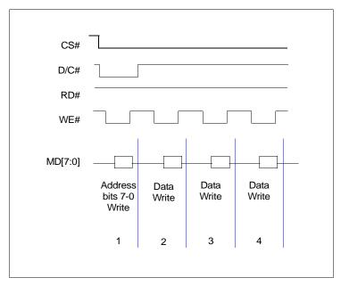
Figure 15-1: Register Write Example Sequence
