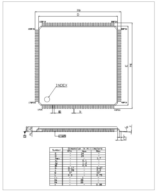
Figure 18-1: S1D13L03 QFP21 176-pin Package
