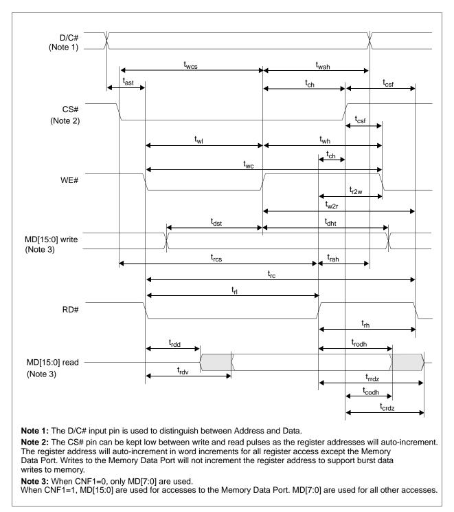
Figure 7-5: Intel 80 Input A.C. Characteristics - 3.3 Volt
