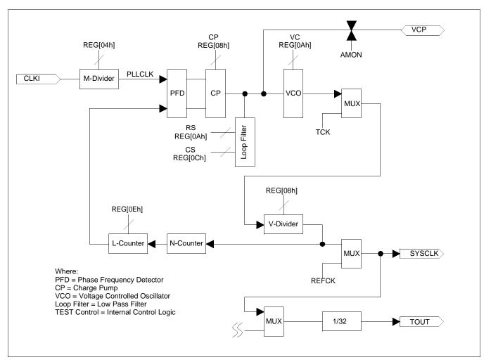
Figure 8-2: PLL Block Diagram
