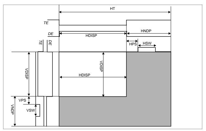
Figure 7-7: Panel Timing Parameters
