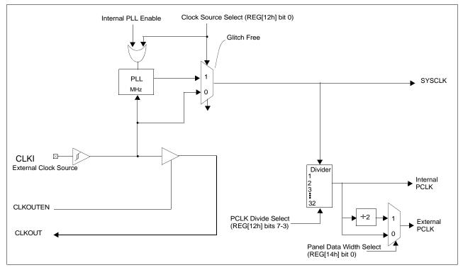
Figure 8-1: S1D13L03 Clock Block Diagram
