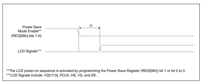
Figure 7-8: TFT Power-On Sequence Timing
