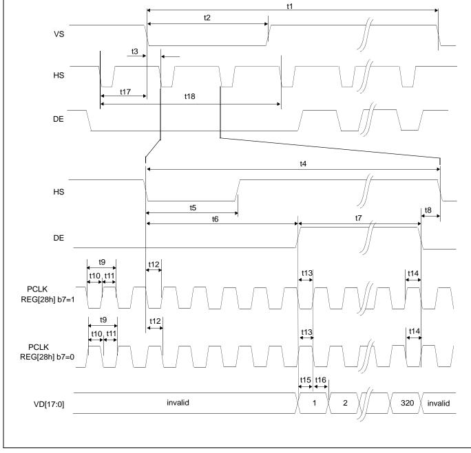
Figure 7-10: 18-Bit TFT A.C. Timing
