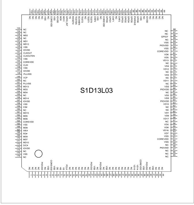
Figure 4-1: S1D13L03 QFP21 176pin Pinout (Top View)
