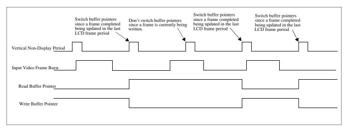
Figure 16-1: Switching of Buffer Pointers
