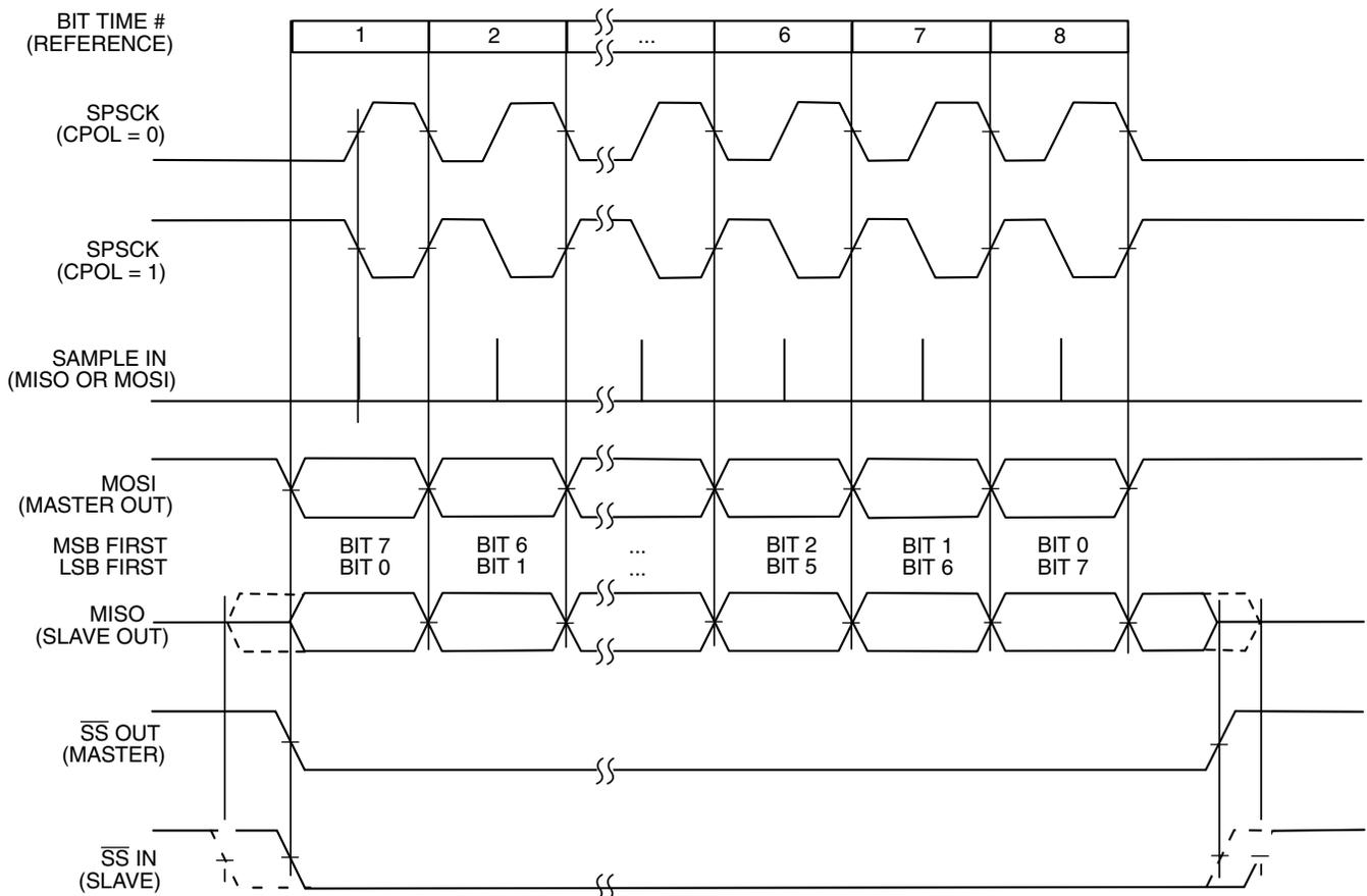
**Figure 16-4. SPI clock formats (CPHA = 0)**
