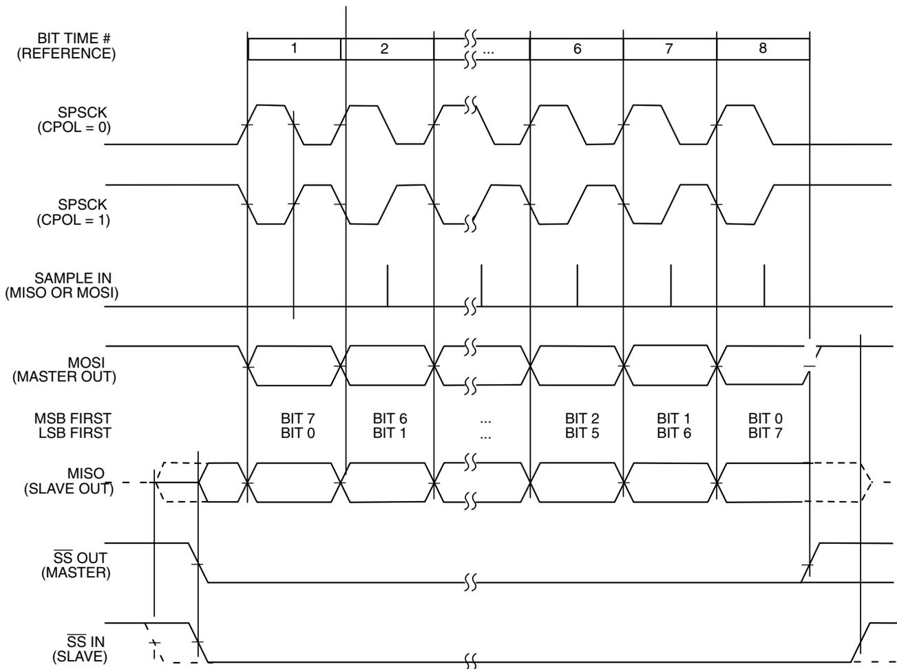
**Figure 16-3. SPI clock formats (CPHA = 1)**
