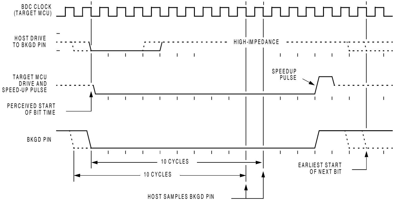
Figure 23-4. BDM target-to-host serial bit timing (logic 0)
