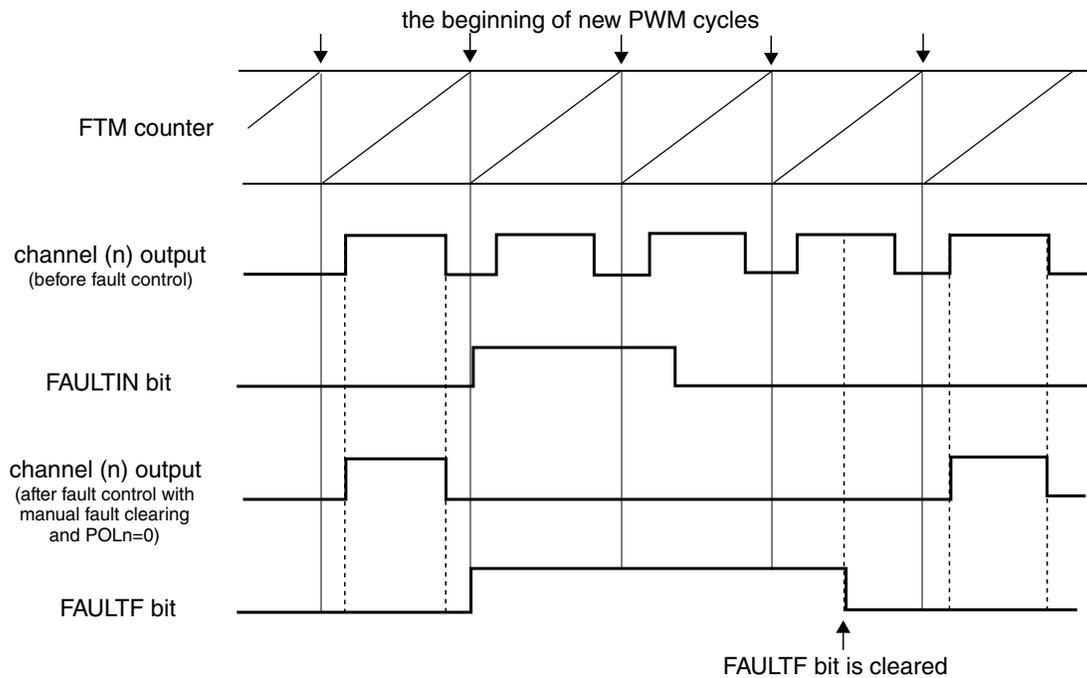
**Figure 12-61. Fault control with manual fault clearing**
