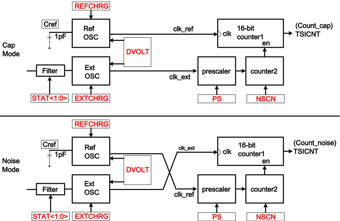
Figure 20-5. TSI noise detection mode block diagram
