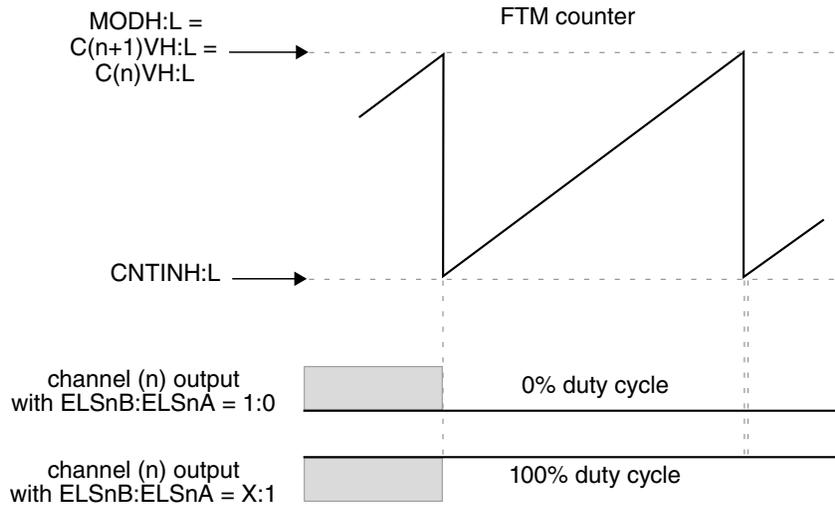
**Figure 12-30. Channel (n) output if  $(C(n)V = C(n+1)V = MOD)$**
