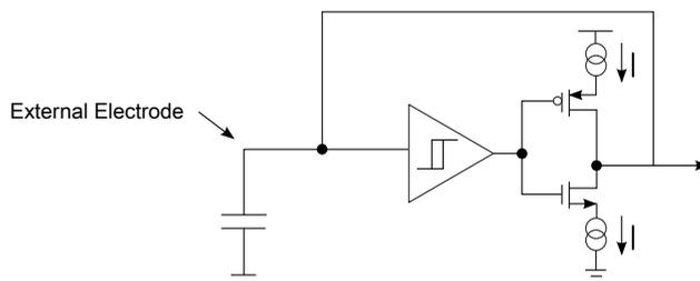
**Figure 20-2. TSI electrode oscillator circuit**
