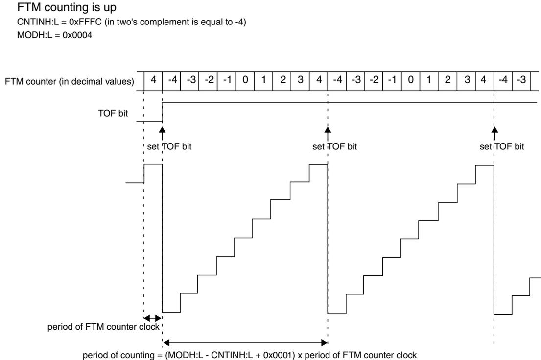
**Figure 12-4. Example of FTM up and signed counting**
