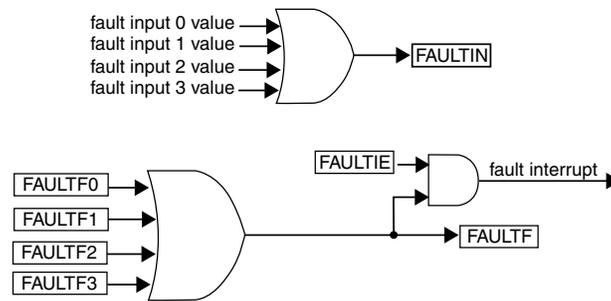
**Figure 12-59. FAULTF and FAULTIN bits and fault interrupt**
