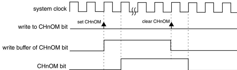
**Figure 12-46. CHnOM synchronization when (SYNCHOM = 0)**
