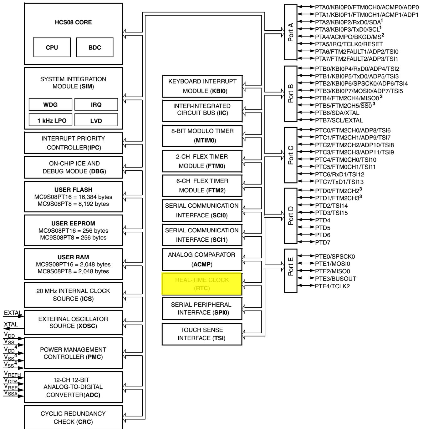
1. PTA2 and PTA3 operate as true-open drain when working as output.
