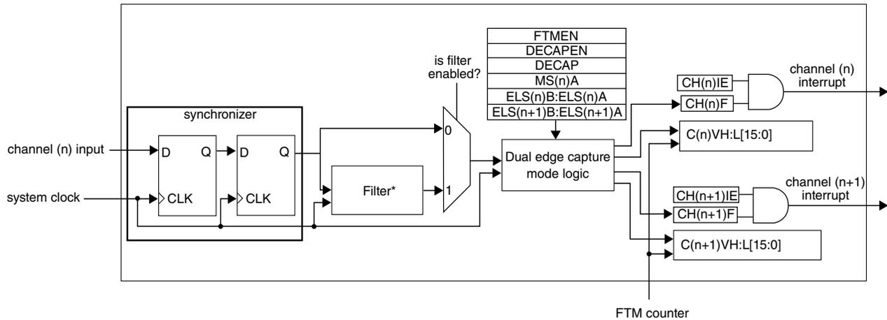
\* Filtering function for dual edge capture mode is only available in the channels 0 and 2
