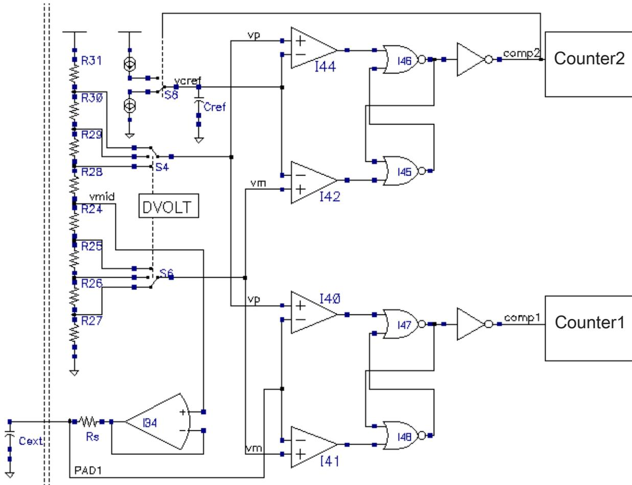
**Figure 20-6. TSI circuit in noise detection mode**
