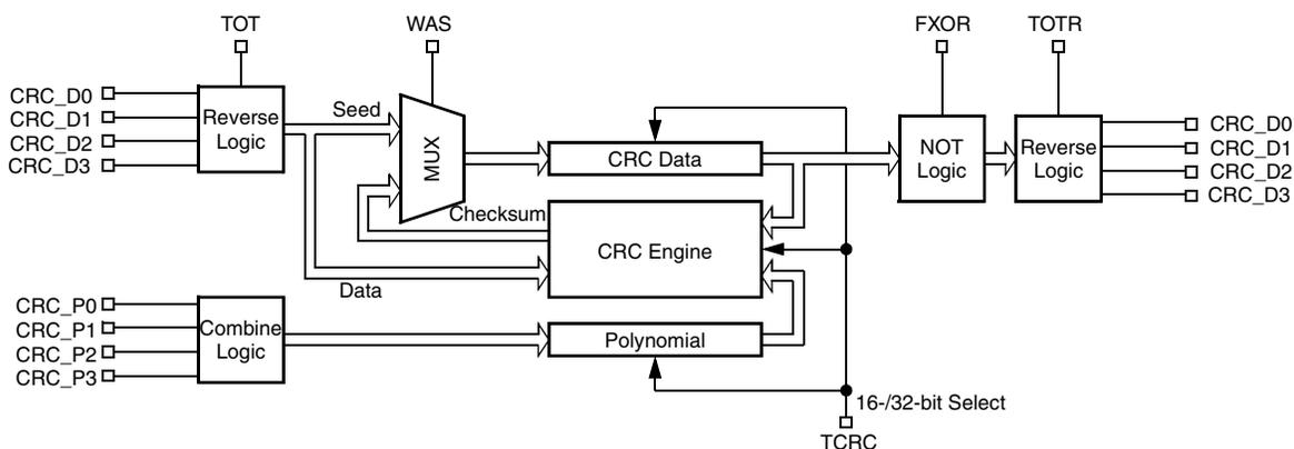
Figure 21-1. Cyclic redundancy check (S08CRC) block diagram
