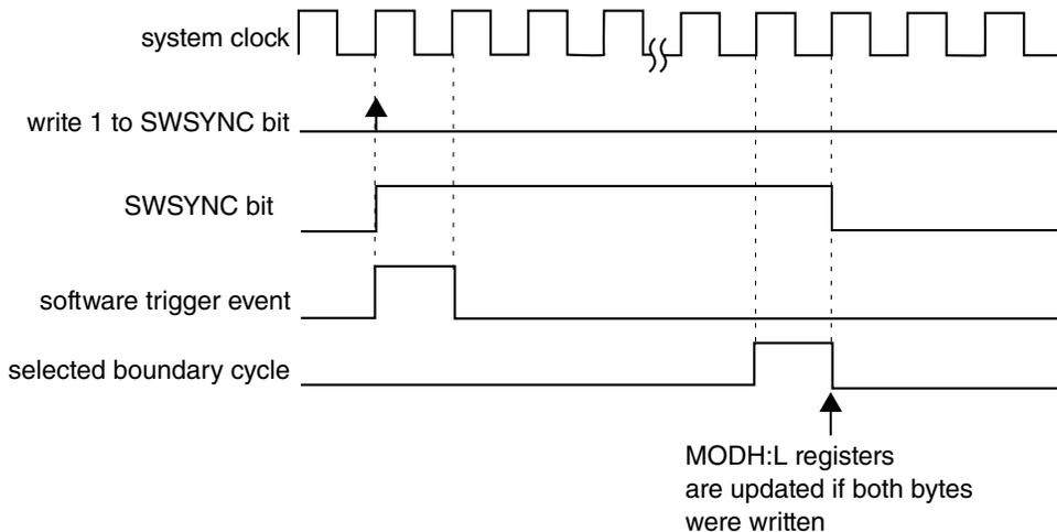
**Figure 12-45. MODH:L synchronization when (PWMSYNC = 1)**
