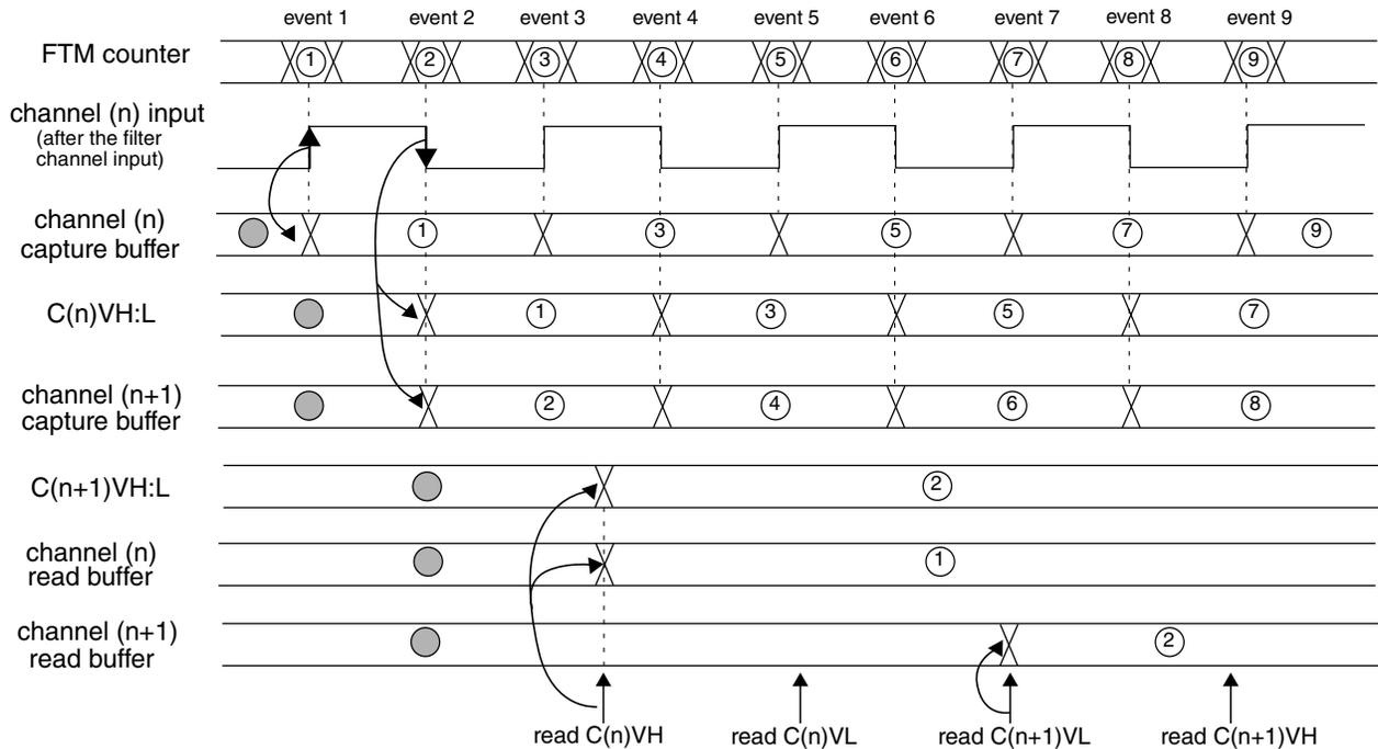
**Figure 12-74. Dual edge capture mode read coherency mechanism**
