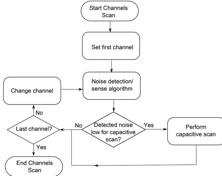
**Figure 20-8. Detection of touch with noise sense and normal capacitive sense flow chart**
