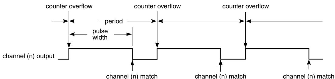
**Figure 12-15. EPWM period and pulse width with  $ELSnB:ELSnA = 1:0$**
