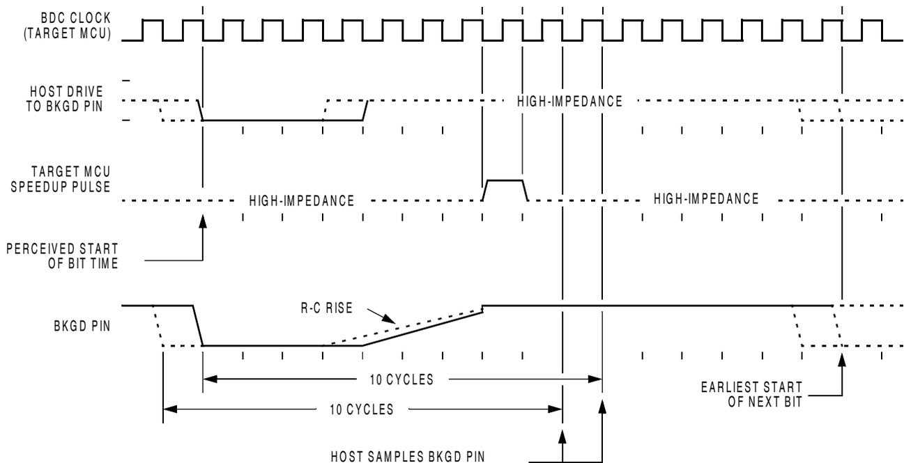
**Figure 23-3. BDC target-to-host serial bit timing (logic 1)**
