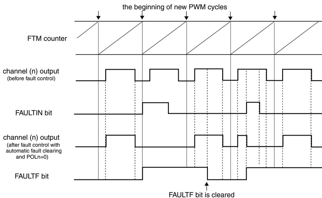
**Figure 12-60. Fault control with automatic fault clearing**
