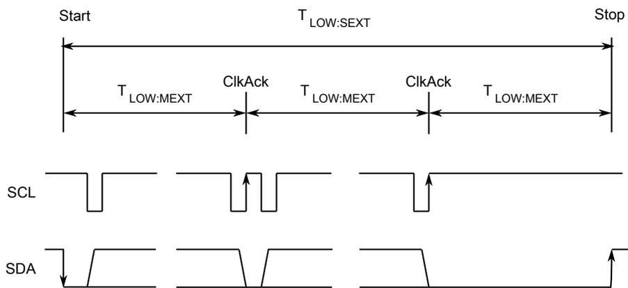
**Figure 17-4. Timeout measurement intervals**
