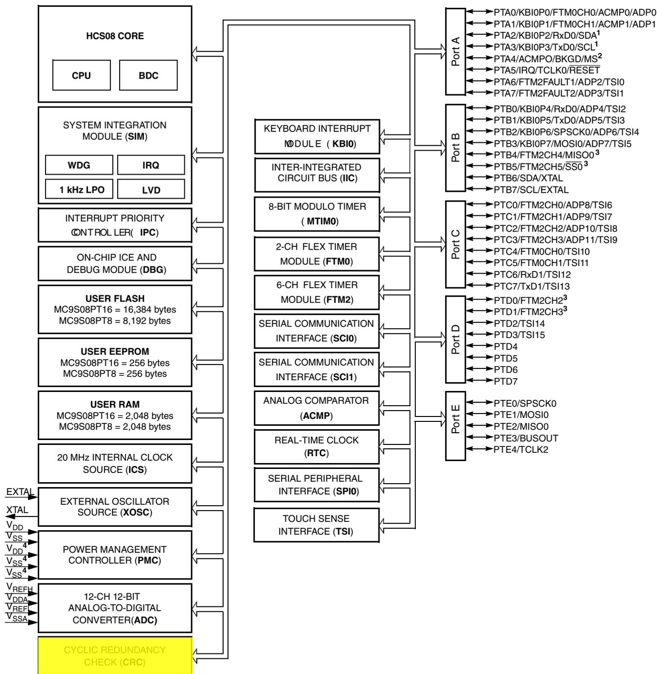
1. PTA2 and PTA3 operate as true-open drain when working as output.
