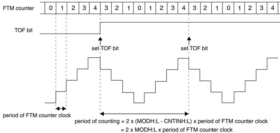
**Figure 12-7. Example of up-down counting when CNTIN = 0x0000**
