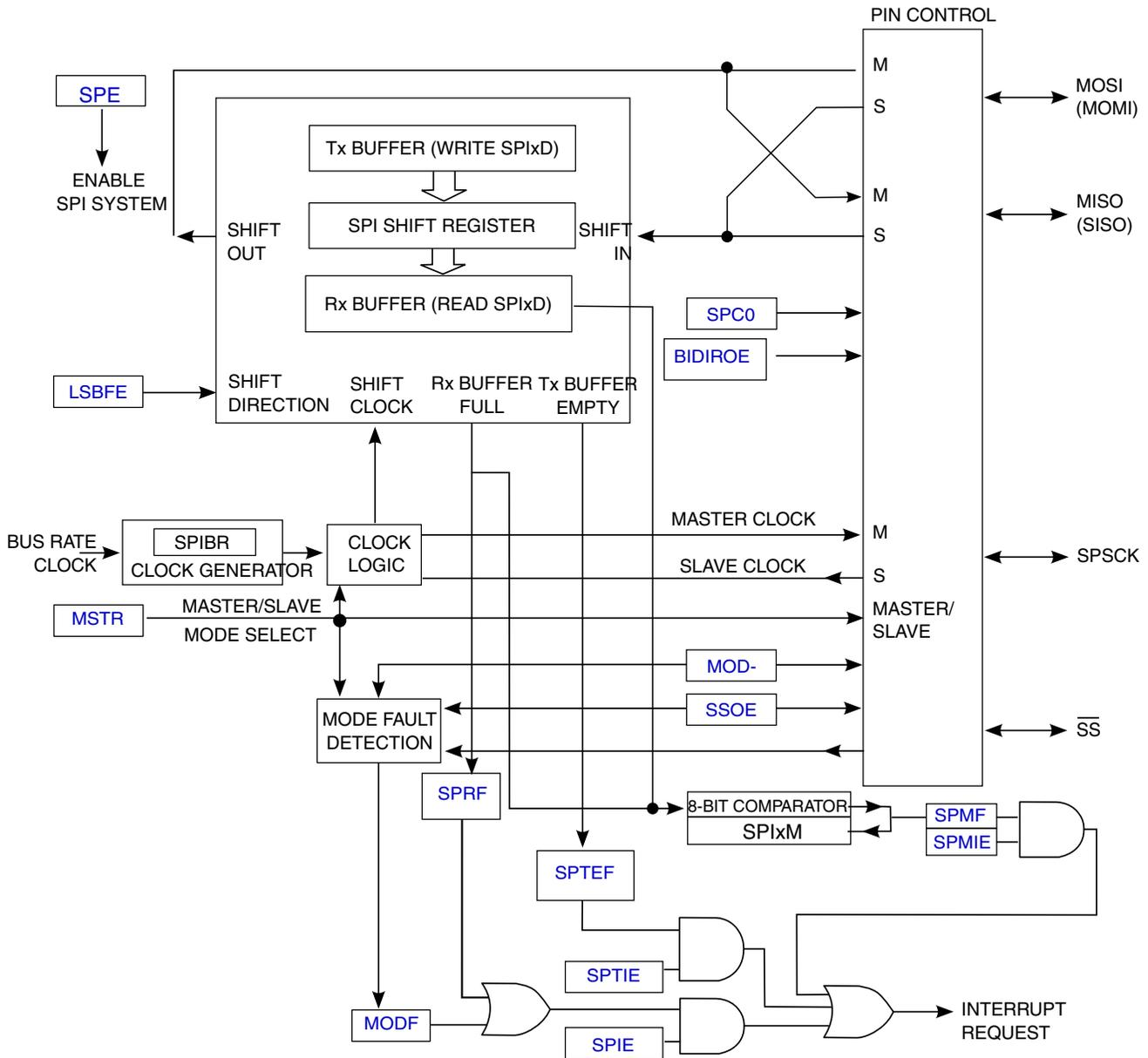
Figure 16-2. SPI module block diagram without FIFO
