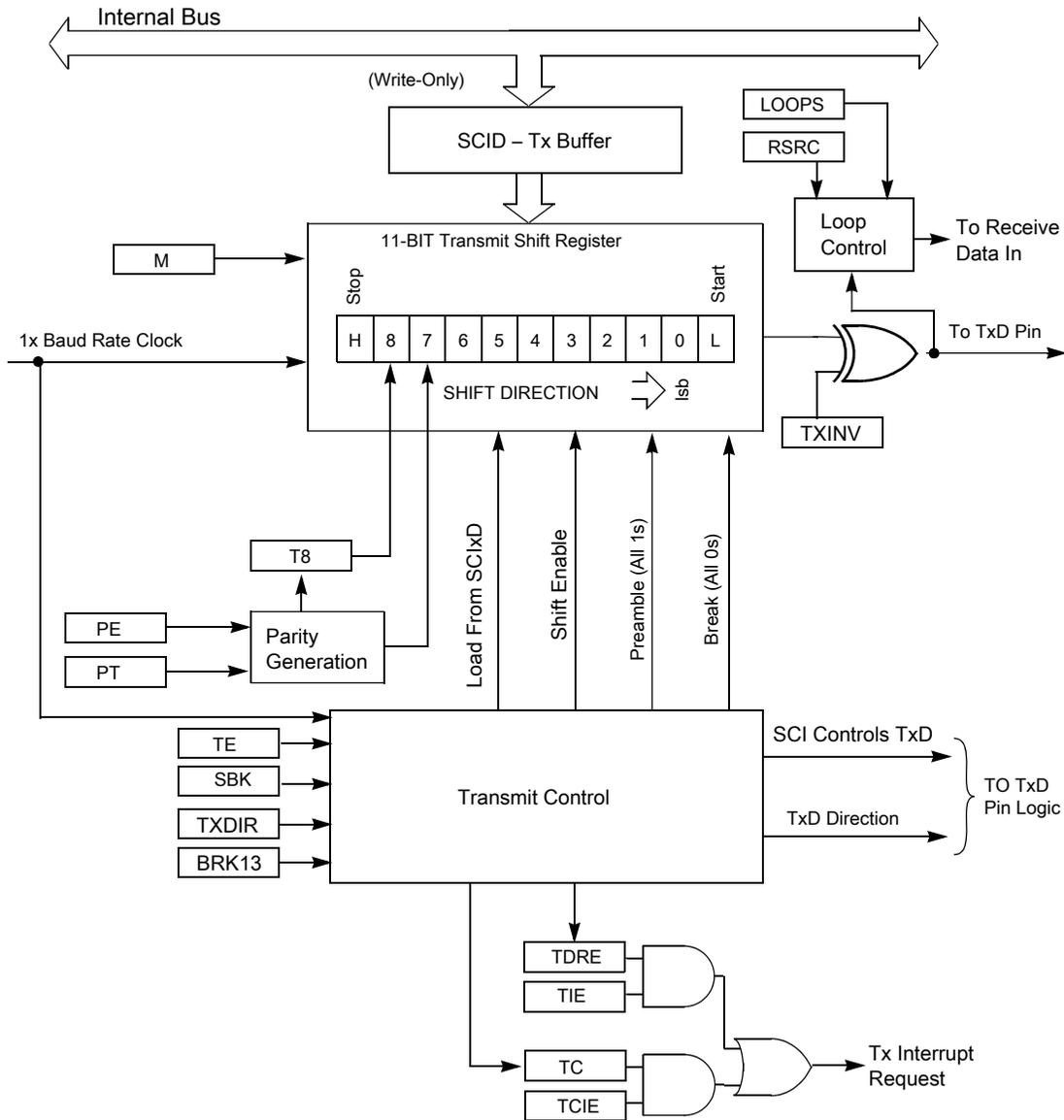
**Figure 15-1. SCI transmitter block diagram**
