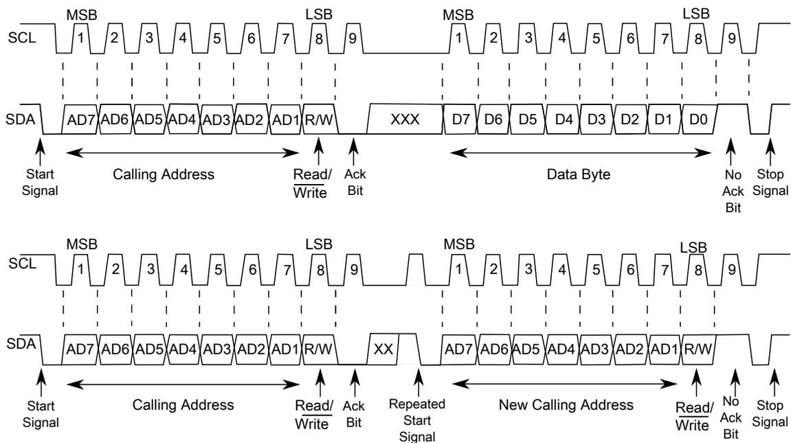
**Figure 17-2. I2C bus transmission signals**
