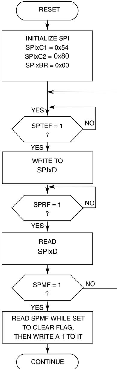
Figure 16-6. Initialization Flowchart Example for SPI Master Device
