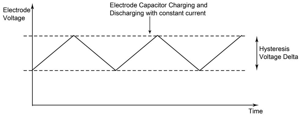
**Figure 20-3. TSI electrode oscillator chart**
