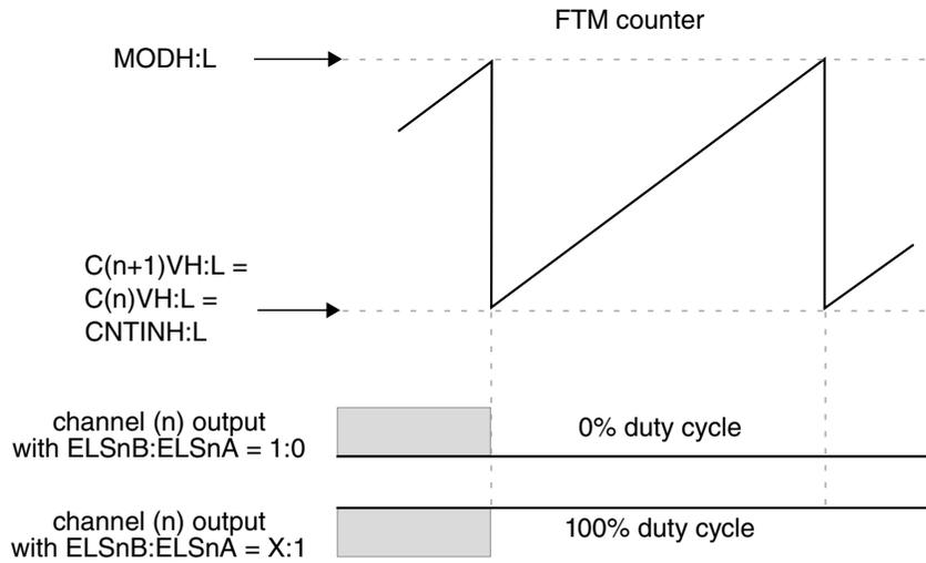
**Figure 12-29. Channel (n) output if  $(C(n)V = C(n+1)V = CNTIN)$**
