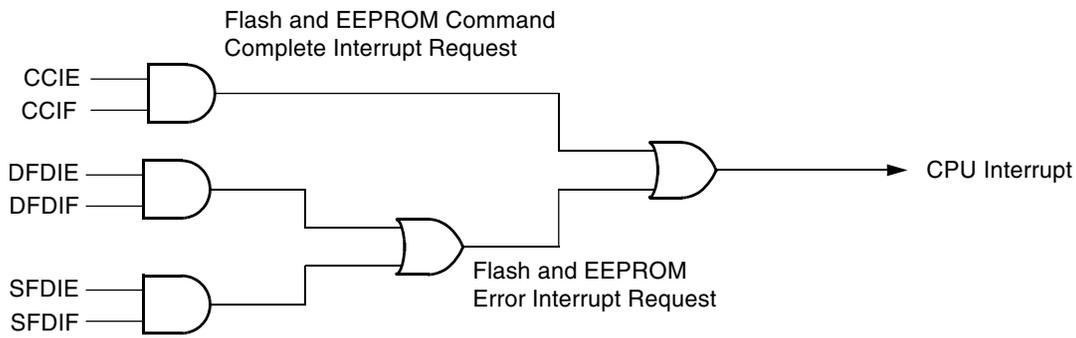
**Figure 4-4. Flash and EEPROM module interrupts implementation**
