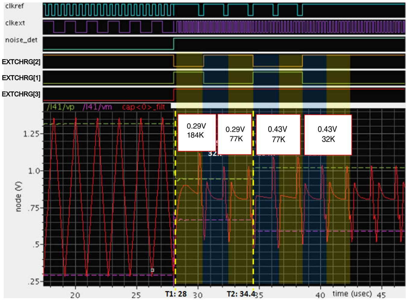
Figure 20-9. TSI noise detection mode waveform
